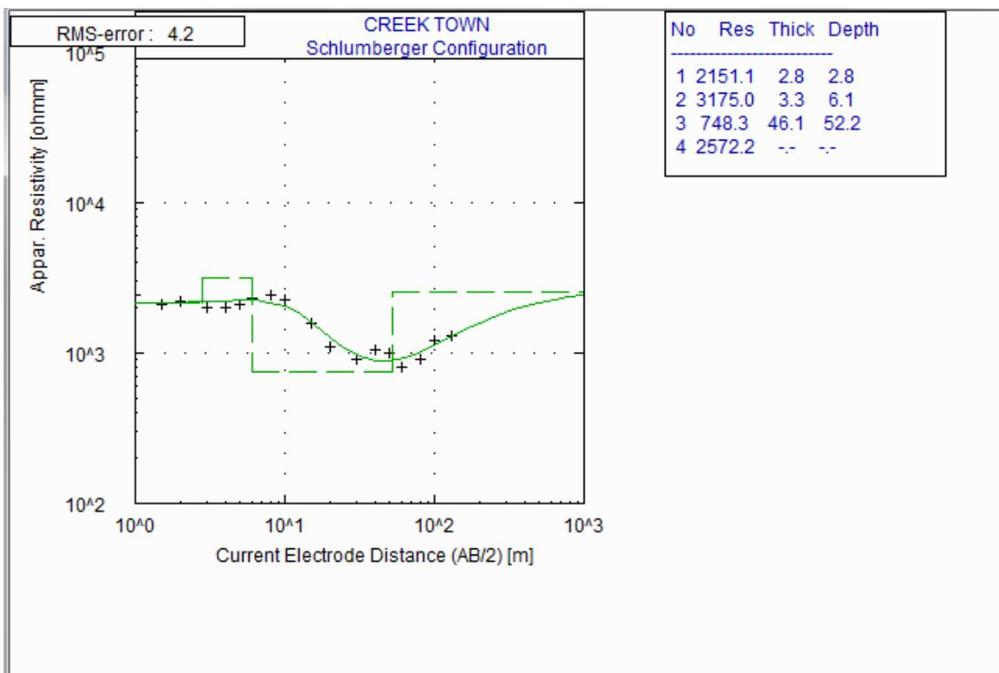
**Figure 3.0:** A Curve (Graph) of Apparent Resistivity against Current Electrode Separation
